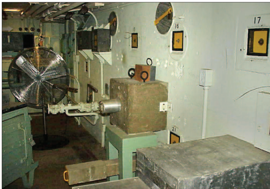
Figure 7. Upper room, where radioisotopes were prepared, after 1945. Radioisotopes were produced by bombarding chemical elements with neutrons from the nuclear chain reactions or fissioning—that occur inside a nuclear reactor. Radioisotopes are used in various applications for medical, industrial, agricultural, military, space, and scientific research. Prepared radioisotopes include iodine-131, phosphorus-32, and carbon-14. The reactor stopped operation in 1963.
